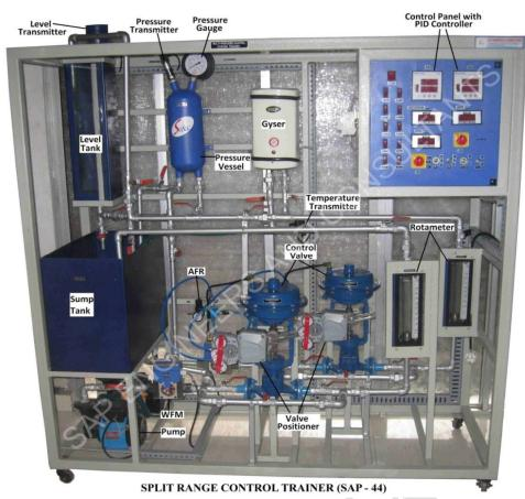
The **Split Range Control Trainer (SAP - 44)** is highly flexible and modular system for studying of Split Range Control Loops (Pressure Control Loop / Level Control Loop) optional in industrial processes.
